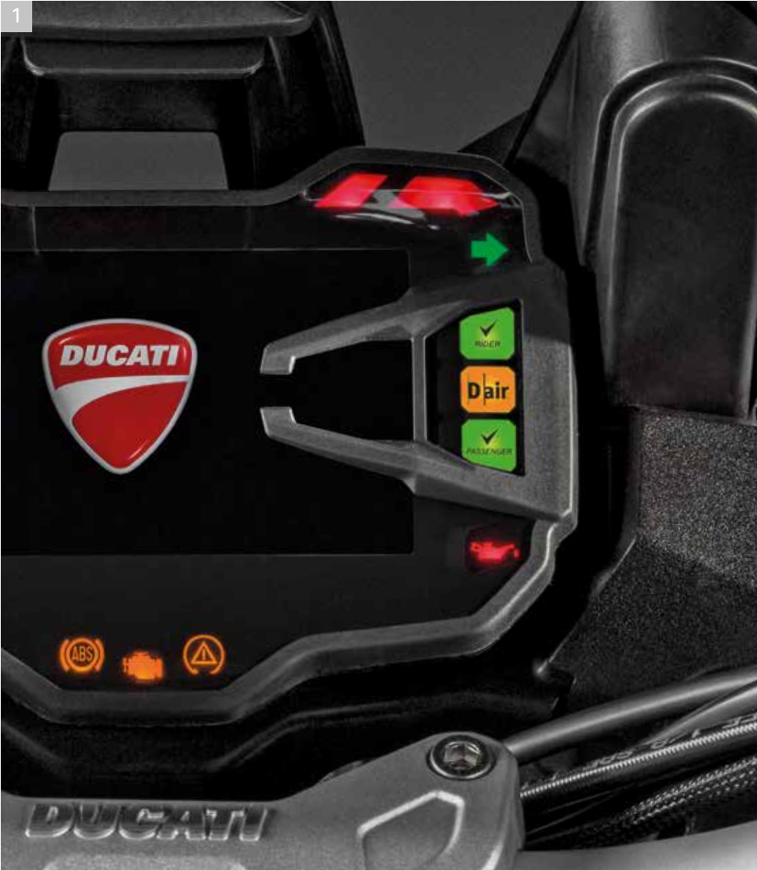
1 D-Air® system warning lights featured on the full-colour TFT display
